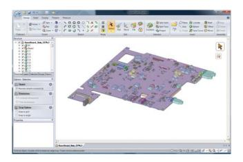
SpaceClaim helps engineers collaborate and converge on key design decisions before sending models out for detailed design in CAD. Working in the context of cross-functional data, such as designing the enclosure around this circuit board, ensures optimal designs up-front
